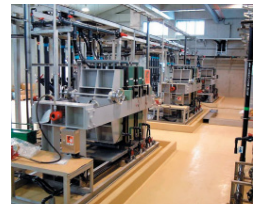
High performance dialyzer “ACILYZER” using ion exchange membranes
