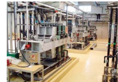
The ACLYZER high performance electro dialyzer based on ion exchange membranes
