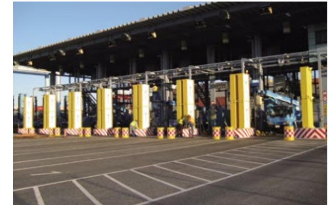
A security gate using neutron detectors to check for nuclear substances
