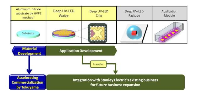
\* Single crystal aluminum nitride growth technology utilizing the hydride vapor phase epitaxy (HVPE) method.
