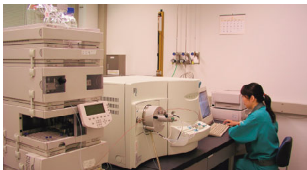
Analyzing organics in wastewater by a liquid chromatograph mass spectrometer system
